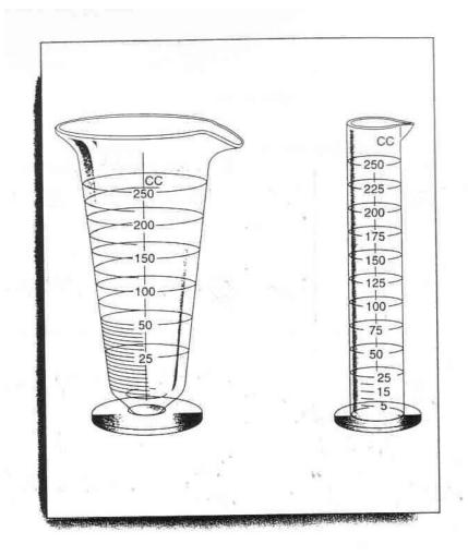
Conical (left) and cylindrical (right) graduates.
