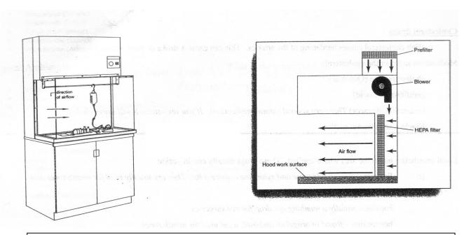
In a **Horizontal Flowhood**, room air is pulled into the back of the hood, through the HEPA filter located in the back. The air passes through the High Efficiency Particulate Air (HEPA) filter where 99.97% of all particles 0.3 microns or larger are removed. The air flows horizontally, from the back of the hood, across the work surface and then out into the room. It is necessary to work at least six inches into the hood due to the mixing of room air and the filtered air.
