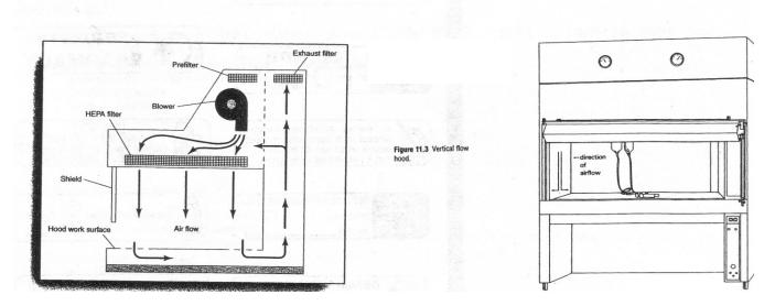
In a **Vertical Flowhood**, the HEPA filter is located in the top of the hood. The air flow moves from the top of the hood straight down onto the work surface. There is a glass shield that pulls down to help prevent splashes from hazardous material onto the worker. This is the hood of choice to work with hazardous materials like chemotherapy agents.
